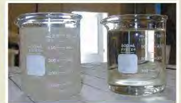
Actual water samples before and after processing with a Beckart system at Midwestern stone cutting facility.
